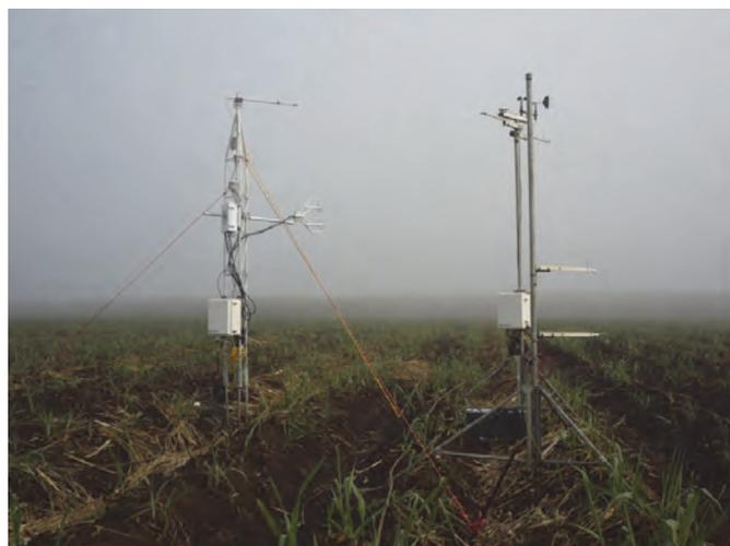
Figure 5. Surface renewal system (*left*) installed in the sugarcane field UVS G1 with the Eddy covariance system (*right*) installed for calibration purposes
