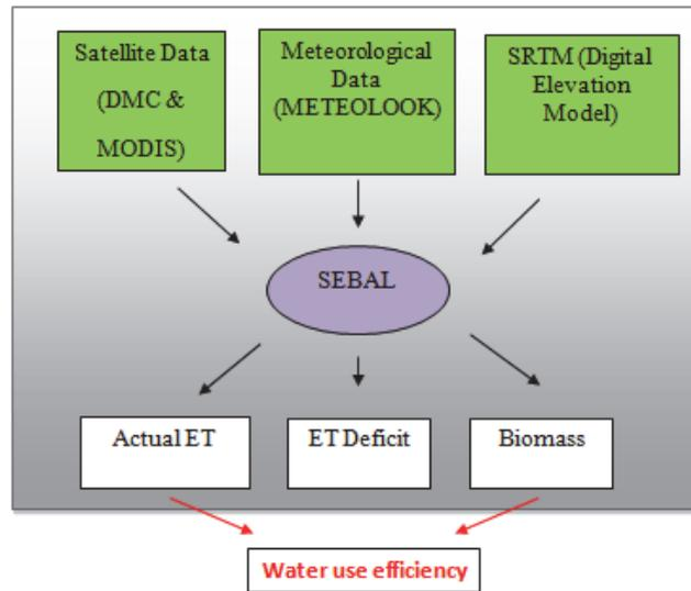
**Figure 9.** Diagram showing important data inputs and outputs (ET, ET<sub>def</sub>, Biomass) from the SEBAL model
