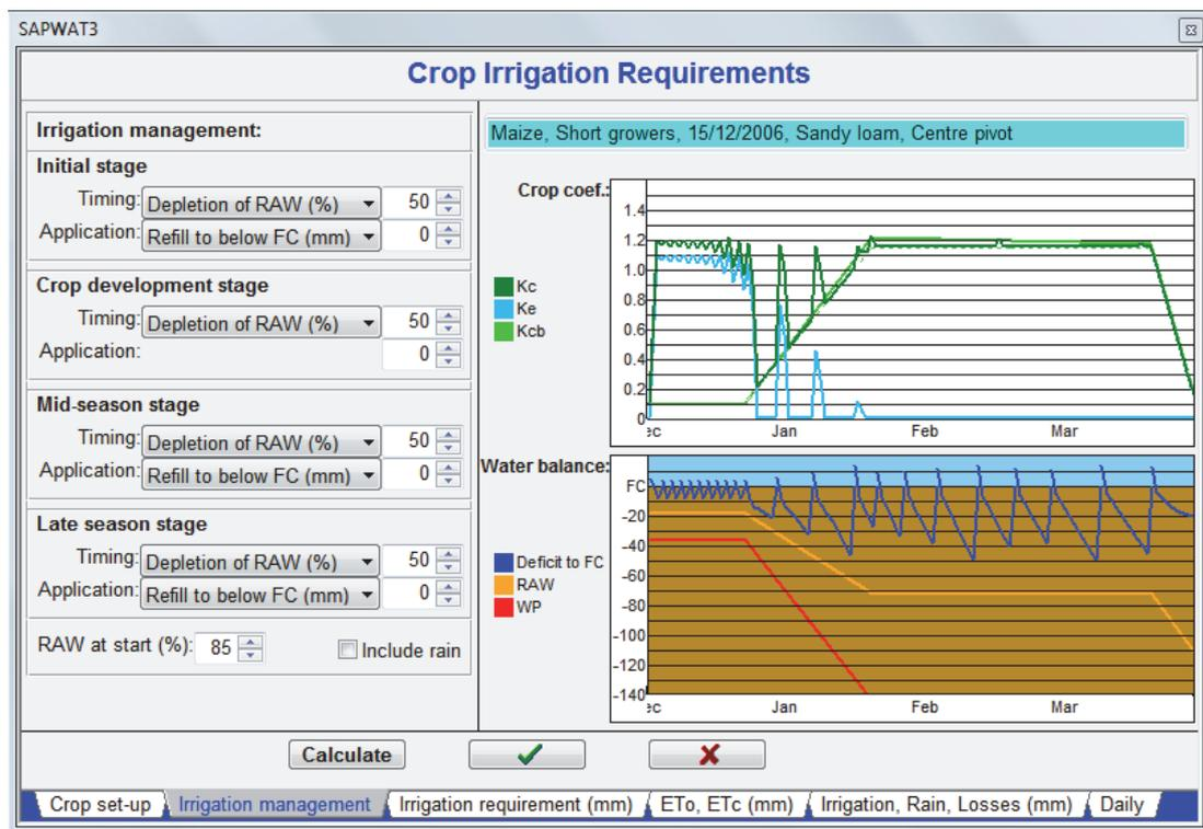
Figure 38. SAPWAT irrigation management interface screen
