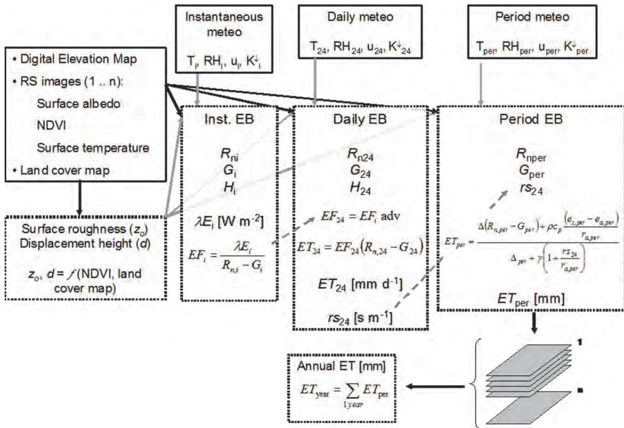
Figure 10. Processing steps performed in the SEBAL model to first derive the surface energy balance and evapotranspiration (ET) at the time of satellite overpass, then for a DAY and lastly for a weekly period
